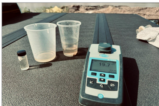
Jar test samples and turbidity meter used on site.
